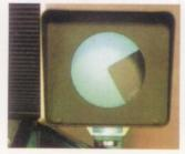
Profile projector, screen diameter 100mm, magnification 10:1 or 20:1 (optional 150mm screen diameter [shown], magnification 20:1, optical angle meter).
