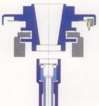
Adaptor spindle for ISO 30-50 tapers (other systems available) equipped with pre loaded high precision needle bearing, disc brake with flexible brake disc 2 x 180° indexing. 4 x 90° on request.
