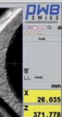
EPRO includes frontal illumination for tip inspection. Visual inspection and measuring of the tool tips are performed in black/white. This enables tool edge checking for possible damage and measuring where required. Magnification 20x and 40x.
