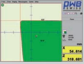
Measuring with floating reticule for quick and easy measurements. The tool to be measured is swivelled past the screen. The cutting edges are automatically identified and measured by the suitable method.
