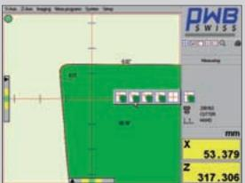
Manual selection of desired measuring method, e.g. line-line to determine intersection coordinates by mouse click.
