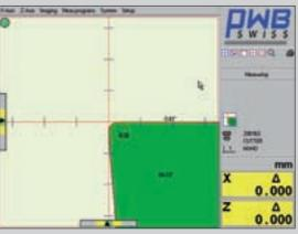
Measuring with fixed reticule for high precision measurements. The cutting edge to be measured is positioned to the electronic reticule using the infinite fine adjustment supported by the graphic adjusting aid.
