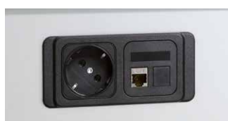
Power module 1 × socket outlet 230 V 2 × RJ45, without network cable, Plug+Play, Cat6
