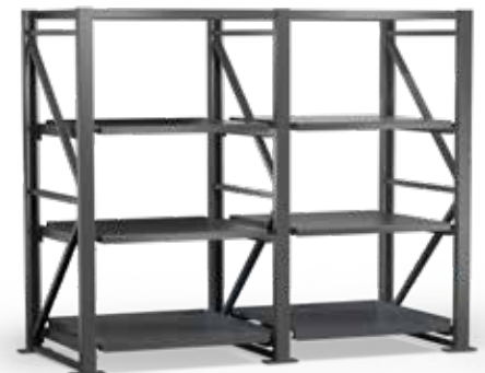
Heavy-duty shelves in a particularly solid design with a load capacity of up to 9 t per shelving unit and 1000 kg per fixed or pull-out frame, secure locking and adaptable in increments of 100 mm
