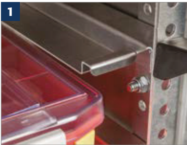
Rails with stops keep CarryLites in place during transportation.
